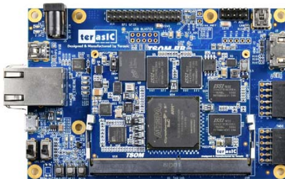
TSOM installed on the TSOM-BB board.
