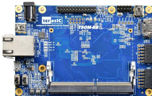
TSOM installed on the TSOM-BB board.
