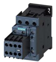
Contactor, AC-3, 15 kW / 400 V, 2 NO + 2 NC, 110 V AC, 50 Hz, 3-pole, Size S0 screw terminal Removable auxiliary switch
