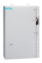
Non-reversing motor starter Size 1 3/4 Three phase full voltage Solid-state overload relay OLRelay amp range 10-40a 220-240/440-480VAC 60HZ coil Combination type 40AMP circuit breaker Enclosure NEMA type 4/12 Water/dust tight for outdoors Extra-wide enclosure
