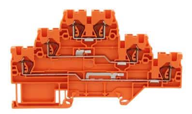
Three-level initiator terminal | Multi-wire terminal, Tension-spring connection, Mounting type: Mounting rail TS 35/7.5, Rated cross-section: 2.5 mm², Width: 5.1 mm, Colour: Orange
