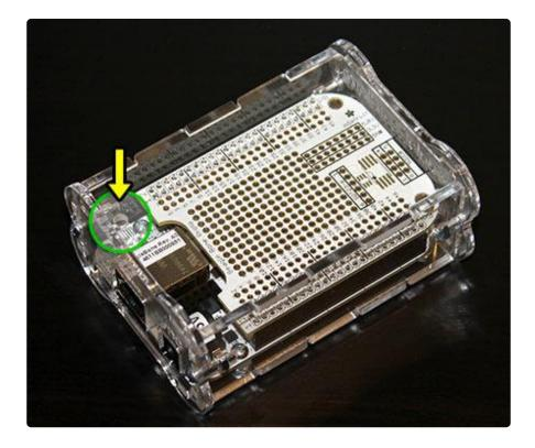
Press the front face flush again and tighten all the screws. Acrylic is brittle, so don't crank these down too hard – finger pressure plus 1/8 turn is sufficient. Insert the microSD card (make sure it goes into the card slot, NOT loose in the case!). Bingo... you're done!
