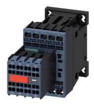
Power contactor, AC-3 16 A, 7.5 kW / 400 V 2 NO + 2 NC, 24 V DC with integrated diode 3-pole, Size S00 Spring type terminal Captive auxiliary switch
