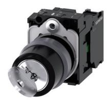
RONIS key-operated switch, 22 mm, round, plastic with metal front ring, lock number SB30, with 2 keys, 2 switch positions O-I, latching, actuating angle 90°, 10:30h/13:30h, key removal O+I, with holder, 1 NO, screw terminal, possible special locks: SB31, 421, 455, with laser labeling, upper case and lower case, always upper case at beginning of line
