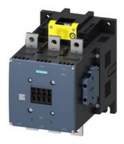
Power contactor, AC-3 400 A, 200 kW / 400 V Coil AC 50/60 Hz and DC 200-277 V x (0.8-1.1) F-PLC input 24 V DC 3-pole size S12 Auxiliary contacts 2 NO + 2 NC Main circuit: Busbar Control and auxiliary circuit: screw terminal
