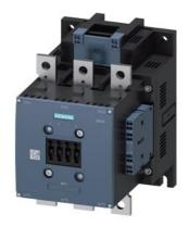
power contactor, AC-3 225 A, 110 kW / 400 V AC (50-60 Hz) / DC operation 220-240 V AC/DC auxiliary contacts 2 NO + 2 NC 3-pole, frame size S10 busbar connections drive: conventional spring-loaded terminal
