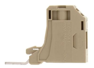
Measurement pick-off terminal, Screw connection, Mounting type: On base, Rated cross-section: 2.5 mm<sup>2</sup>, Width: 5.9 mm, Colour: Beige
