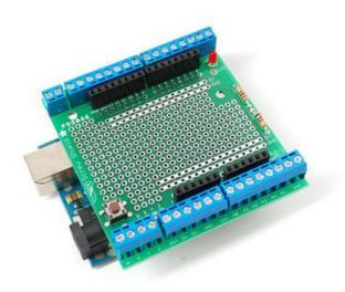
That's it! You can now insert the headers into the Arduino and start using the shield!
