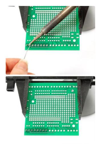
And solder the pins to the pads. Use plenty of solder so that you get the pads completely filled.
