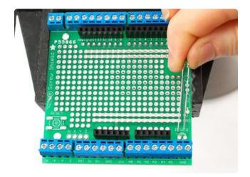
Next we'll place the two LEDs. The first LED is the green-colored one. This will tell us when the Arduino and shields are powered.
