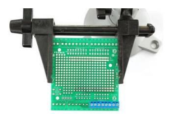
Get ready by putting the PCB in a vise. Then you can start by placing one of the 8piece terminal blocks in the "Analog" breakout area.
