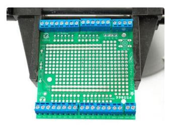
Place the remaining terminal blocks, checking again that they face the right direction!
