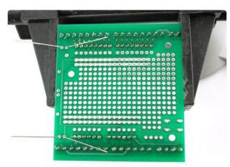
You can bent the LED leads out of the way to keep the LEDs flat against the PCB.
