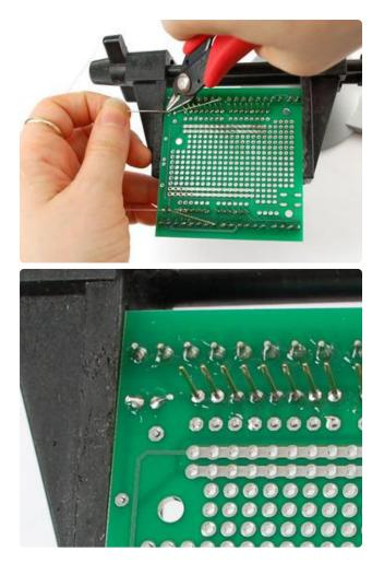
Use the diagonal cutters to clip the long LED legs. They should be cut just above the solder joint.
