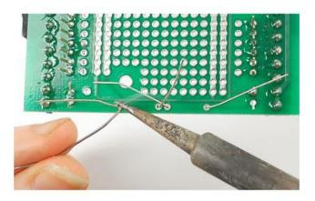
Solder and clip the two resistors.
