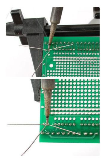
Solder both LEDs in place.
