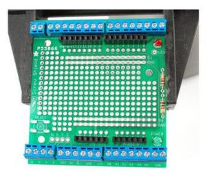
Next we will place the two 1.0Kohm resistors. These resistors are used to set the brightness of the LEDs. If you want brighter LEDs you can substitute 220 ohm resistors. If you want dimmer LEDs, you can use 4.7Kohm.
