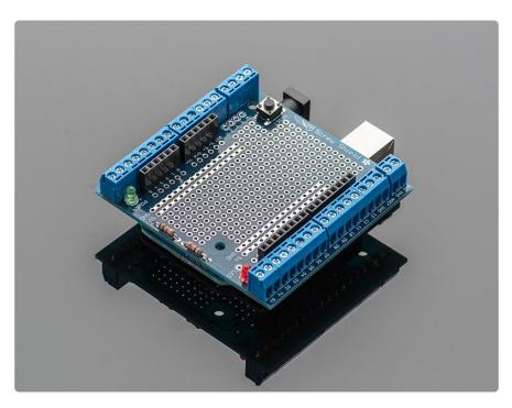
The shield even comes with <u>stacking headers</u>, () which let you plug another shield on top! As shown here, a data logging shield is stacked onto the proto-screwshield.
