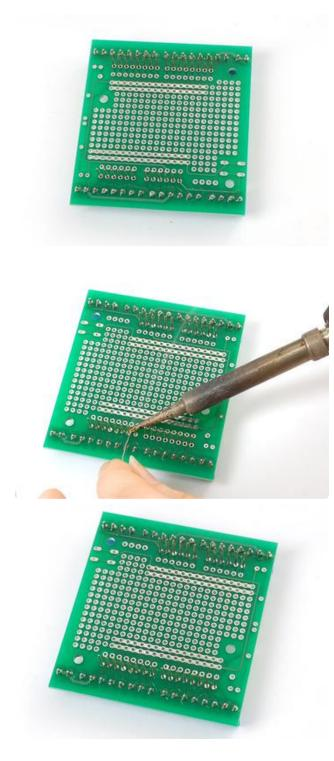
Flip over the PCB, you can lay it down on a table again, just make sure that all the headers are sticking out straight.
