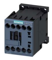
Power contactor, AC-3 9 A, 4 kW / 400 V 1 NO, 125 V DC 3-pole, Size S00 screw terminal
