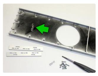
The spine, middle separator and the frame sides are joined using 1/2" #4-40 screws and nuts (20 total). About \$3. The top and bottom edges will be added shortly.
