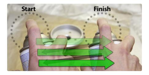
Avoid clogs: when done, clear the nozzle by inverting the can and spraying until just air comes out...or some newer nozzle designs work fine just wiping with a rag.
