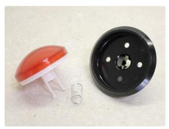
The button then slides out the front of the bezel. Don't lose that spring!
