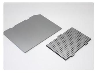
The speaker grille required its own set of hoops to jump through: all those tiny holes would be time-consuming and error prone (laser-cut holes tend to stick in place). Instead, a scrap of black acrylic was painted before cutting, then the laser was used to etch the surface and reveal the black plastic underneath those spots before the final perimeter cut.
