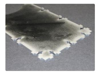
Because T-slot construction was used, the edges of the main spine need special attention. They'll be poking through the frame sides, so the edges of this one piece were also painted to match.
