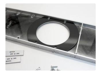
This spacer ring makes the unit feel more solid, so it doesn't cave in when the button is pressed. Note that it's not quite symmetrical — there's a definite "up" and "down" due to the T-slots.
