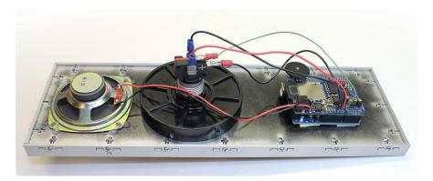
The Wave Shield includes solder holes adjacent to each Arduino header pin, allowing wires to be added. Remove the shield from the Arduino, insert wires from above and solder on the underside. The following connections are made:
