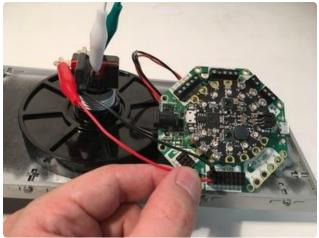
Connect the red and black button wires to the Signal and GND ports.
