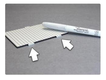
The edge tabs on the grille needed to be painted too, but spraying would ruin the engraved "holes." A silver Sharpie marker did the trick...but you could also spray a little paint into a disposable cup and dab it on with a brush or Q-tip.
