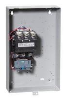
Non-reversing motor starter, Size 3, Three phase full voltage, Solid-state overload relay, OLR amp range 25-100A, Non-combination type, Enclosure type 1, Indoor general purpose use, Standard width enclosure
