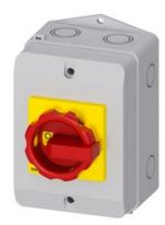
SENTRON, Switch disconnector 3LD, emergency switching-off switch, 3-pole, Iu: 16 A, operating power / at AC-23 A 400 V: 7.5 kW, Molded plastic encapsulation for inch cable gland, rotary operating mechanism, red/yellow
