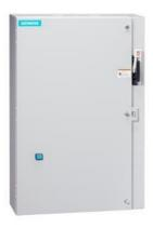
Non-reversing motor starter, Size 2 1/2, Three phase full voltage, Solidstate overload relay, OLR amp range 25-100A, 24VDC coil, Combination type, 60A fusible disconnect, 60A/600V fuse clip, Enclosure NEMA type 1, Indoor general purpose use, Extra-wide enclosure
