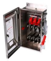
Siemens Low Voltage Circuit Protection Heavy Duty Safety Switches. Type: ENCLOSED, SAFETY SWITCH Std: UL V. Rating: 600V A. Rating: 60A Wattage: 3W No. Of Poles: 3P F. Rating: 60Hz Action: SINGLE THROW Material: SS Enclosure: TYPE 4X. 2-3 point mounting holes. Insulation: YES O. Cycles: 10000 O. Temperature: (-20F-120F) AMBIENT TEMPERATURE Environmental Conditions: INDUSTRIAL CORROSIVE RESISTANCE
