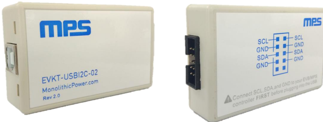
Figure 3: EVKT-USBI2C-02 Communication Interface
