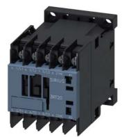
power contactor, AC-3 12 A, 5.5 kW / 400 V 1 NC, 100 V AC, 50 Hz 100-110 V, 60 Hz, 3-pole Size S00 ring cable lug connection
