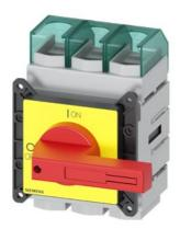
SENTRON, Switch disconnector 3LD, emergency switching-off switch, 3-pole, Iu: 160 A, operating power / at AC-23 A 400 V: 75 kW, front-mounted, knob-operated mechanism, red/yellow, 4-hole mounting of the handle
