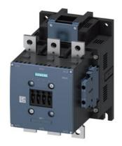
Contactor, AC-1, 400 A/690 V/40 °C, S10, 3-pole, 575-600 V AC/DC, with varistor, 2 NO+2 NC, Connection rail/ screw terminal
