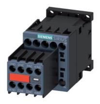
Power contactor, AC-3 9 A, 4 kW / 400 V 2 NO + 2 NC, 230 V AC, 50/60 Hz 3-pole, Size S00 Screw terminal Captive auxiliary switch
