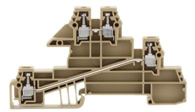
Three-wire installation terminal, Screw connection, Mounting type: Mounting rail TS 35/7.5, Rated cross-section: 2.5 mm<sup>2</sup>, Width: 6 mm, Colour: Beige
