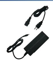
Use only the power cord provided with the unit (4 ft - 1.2m) or equivalent UL approved type SPT-2, SVT, or SJT 18/3 AWG 100-240 VAC, 1 Amp 60°C:
