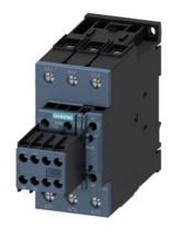
Power contactor, AC-3 65 A, 30 kW / 400 V 2 NO + 2 NC, 175-280 V AC/DC with varistor 3-pole, size S2 screw terminals
