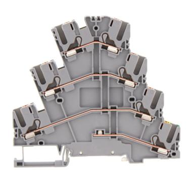
Three-level initiator terminal |Multi-wire terminal, Push-in connection, Mounting type: Mounting rail TS 35/7.5, Rated cross-section: 2.5 mm², Width: 5.1 mm, Colour: Grey
