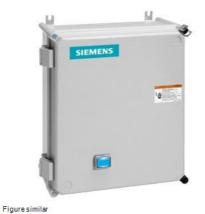
Non-reversing motor starter, Size 0, Three phase full voltage, Solid-state overload relay, OLR amp range 0.75-3.4A, Non-combination type, Enclosure type 4X fiberglass, Water/dust tight noncorrosive, Standard width enclosure
