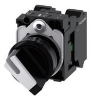
Selector switch, illuminable, 22 mm, round, plastic, white, selector switch, short, 2 switch positions O-I, latching, 10:30h/13:30h, with holder, 1 NO, 1 NC, spring-type terminal, with laser labeling, upper case and lower case, always upper case at the beginning of the word
