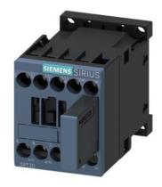
power contactor, AC-3 9 A, 4 kW / 400 V 1 NC, 24 V DC 0.7-1.25\* US, with varistor plugged on, 3-pole, size S00, screw terminal not expandable with auxiliary switch
