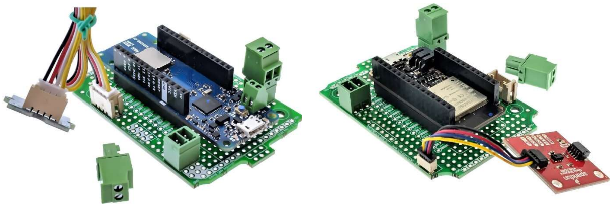
Pic.6. Grove and JST sensor boards connection example
