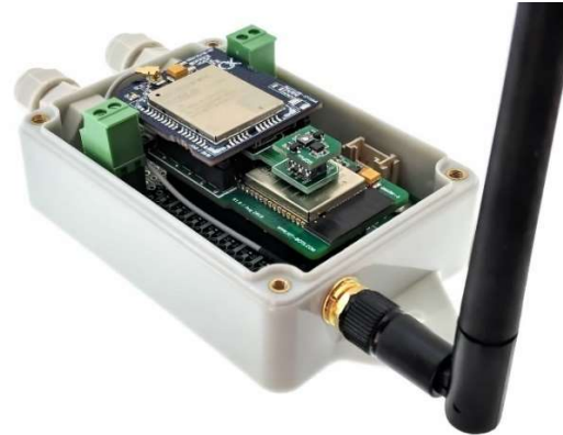
Pic. 15. NB-IOT WiFi / BT / BLE DIY air quality controller
