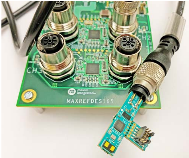
Figure 2. The MAXREFDES171# reference design (right) connected to the MAXREFDES165# IO-Link master reference design (left) for verification.
