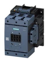
power contactor, AC-3 115 A, 55 kW / 400 V AC (50-60 Hz) / DC operation 21-27.3 V AC/DC auxiliary contacts 2 NO + 2 NC 3-pole, frame size S6 with box terminals drive: electronic with PLC interface 24 V DC screw terminal
