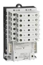
Electrically held lighting contactor, (convertible to mech. held), Amp rating 30A (tungsten 20A), 6 N.C. / 0 N.O. poles, 230-240V 60Hz/220V 50Hz coil, Non-combination type, Enclosure NEMA type (open), No enclosure
