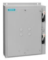
Duplex starter w/ alternator, Size 1, Three phase full voltage, Solid-state overload relay, OLR amp range 3-12A, 110V 50Hz / 120V 60Hz coil, Combination type, Two 10A circuit breakers, Encl NEMA type 4X 304 S-Steel, Water/dust tight noncorrosive
