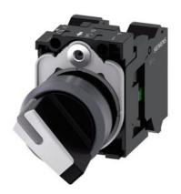
Selector switch, illuminable, 22 mm, round, plastic with metal front ring, white, selector switch, short, 2 switch positions O-I, latching, actuating angle 90°, 10:30h/13:30h, with holder, 1 NO, 1 NC, spring-type terminal, Z=20-unit packaging
