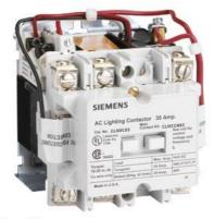
Mechanically held lighting contactor, Contactor amp rating 30A, 0 N.C. / 3 N.O. poles, 277VAC 60HZ coil, Non-combination type, Enclosure NEMA type (open), No enclosure
