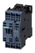
Traction contactor, AC-3 17 A, 7.5 kW / 400 V 1 NO + 1 NC with electronic drive 24 V DC, 0.7-1.25\* US, with integrated varistor, 3-pole, Size S0, Spring-type terminal
