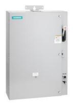
Pump control panel, Size 3 1/2, Three phase full voltage, Solid-state overload relay, OLR amp range 50-200A, 110V 50Hz / 120V 60Hz coil, Standard type contactor, 200A fusible disconnect, 200A/600V fuse clip, HOA Sel Sw. <(>&<)> Start P.B., Enclosure NEMA type 3/3R, Weather proof outdoor use
