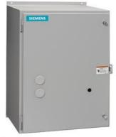
Mechanically held lighting contactor, Contactor amp rating 200A, 0 N.C. / 3 N.O. poles, 277VAC 60HZ coil, Non-combination type, Enclosure NEMA type 12, Dust/drip proof for indoors
