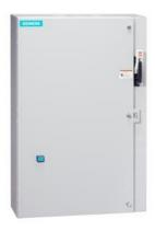
Non-reversing motor starter, Size 4, Three phase full voltage, Solid-state overload relay, OLR amp range 50-200A, Combination type, 200A fusible disconnect, 200A/250V fuse clip, Enclosure NEMA type 1, Indoor general purpose use, Standard width enclosure
