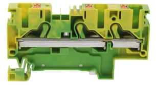
Protective earth terminal, Push-in connection, Mounting type: Mounting rail TS 35/7.5, Rated cross-section: 6 mm<sup>2</sup>, Width: 8.1 mm, Colour: Green-yellow
