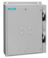
Duplex starter w/ alternator, Size 1 3/4, Three phase full voltage, Amb compensate bimetal OLrelay Contactor amp rating 40Amp 110V 50HZ / 120V 60HZ coil, Combination type, Two 60A disconnect switches Enclosure NEMA type 12, Dust/drip proof for indoors
