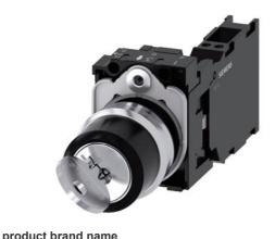
RONIS key-operated switch, 22 mm, round, metal, shiny, lock number SB30, with 2 keys, 2 switch positions O-I, latching, actuating angle 90°, 10:30h/13:30h, key removal O+I, with holder, 1 NO+1 NC, spring-type terminal, possible special locks: SB31, 421, 455, upper case and lower case, always upper case at beginning of line
