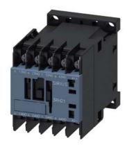
Coupling contactor relay, 4 NO, 24 V DC, 0.7  $\dots$  1.25\* US, with integrated suppressor diode, Size S00, Ring cable lug connection, suitable for PLC outputs
