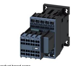
Power contactor, AC-3 9 A, 4 kW / 400 V 2 NO + 2 NC, 24 V DC 3-pole, Size S00 Spring-type terminal connected to varistor
