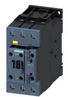
contactor, AC-3, 40 A/400 V/60  $^\circ C$  S2, 3-pole, 83-150 V AC/DC, F-PLC-IN, with varistor, 1 NC, screw terminal
