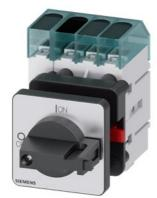
Load disconnector 3LD3, lu 63 A Main switch 3-pole + N Rated operating capacity at AC-23 A at 400V 22.0 kW Front plate mounting Basic switch with Central hole mounting 22.5mm Toggle drive black 48x48 mm
