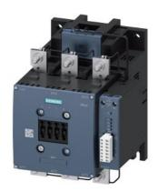
power contactor, AC-3 225 A, 110 kW / 400 V AC (50-60 Hz) / DC operation 96-127 V AC/DC auxiliary contacts 1 NO + 1 NC 3-pole, frame size S10 busbar connections drive: electronic with PLC / SIMOCODE - interface and remaining lifetime signal
