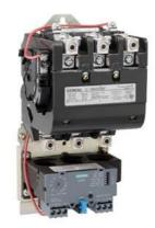
Non-reversing motor starter Size 3 1/2 Three phase full voltage Solid-state overload relay OLRelay amp range 50-200A 24VAC 50-60HZ coil Combination type No enclosure
