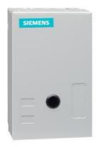
Electrically held lighting contactor, Contactor amp rating 30A, 0 N.C. / 3 N.O. Poles, 110VAC 50HZ/120VAC 60HZ coil, Non-combination type, (no disconnect device), Enclosure NEMA type 1, Indoor general purpose use
